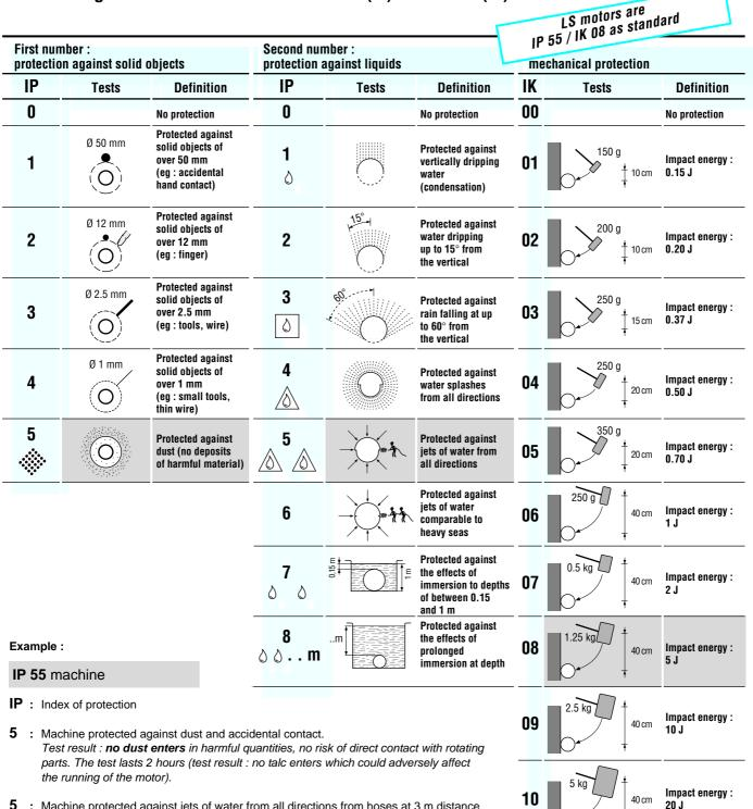
5 : Machine protected against jets of water from all directions from hoses at 3 m distance with a flow rate of 12.51 / min at 0.3 bar. The test lasts 3 minutes (*test result* : *no damage from water* projected onto the machine).
